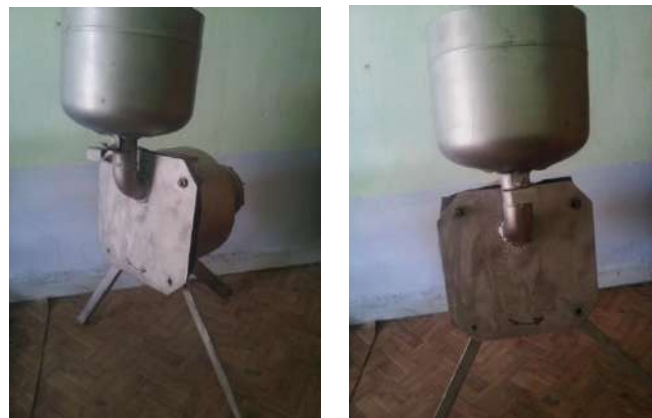
Figure 8. Hammer mill (under laboratory conditions)
