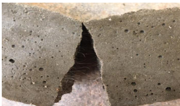
1.1-rasm. Mayda donali betondagi polipriopilen tolalari
