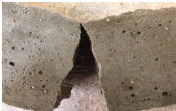
1.4-rasm. Mayda donali betondagi bazalt tolalari
