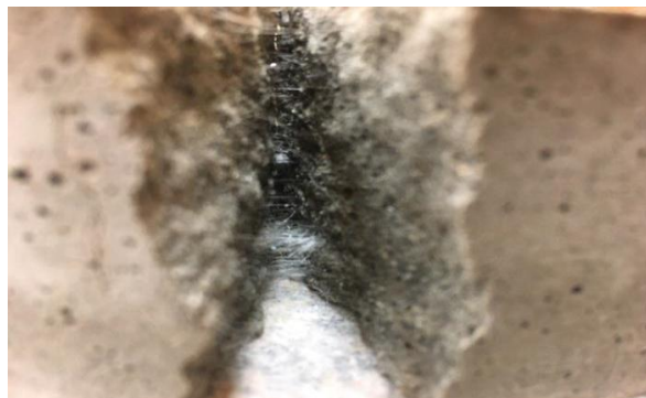
1.1-rasm. Mayda donali betondagi polipriopilen tolalari
