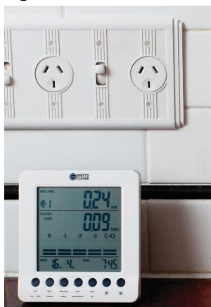
Typical in-home display, indicating present rate of electricity use (watts), recent use (kWh) and rate of expenditure at current use
