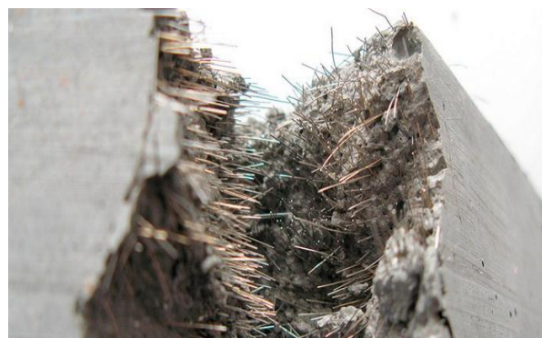
1.4-rasm. Mayda donali betondagi bazalt tolalari
