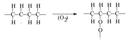
The resulting peroxide radical is unstable and takes a hydrogen atom from another polyethylene molecule. Thus, the oxidation reaction of polyethylene turns into a chain reaction [9].
