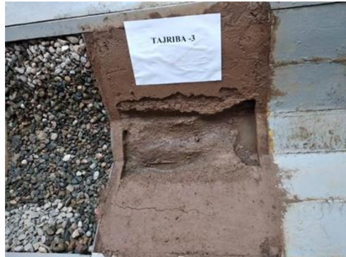
Fig. 1.4. Scour of cohesive soil in the lower pool
